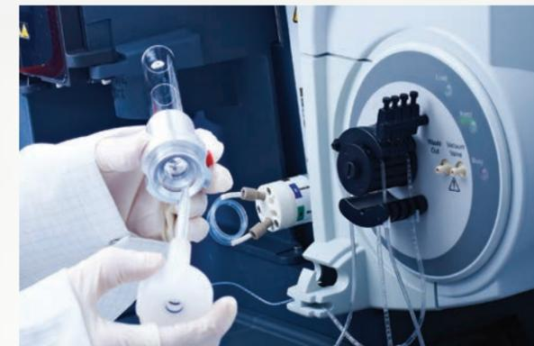
The user-friendly sample introduction system with push-fit connections ensures rapid assembly and disassembly for cleaning and maintenance. Alternative sample introduction components can be added to increase the speed of analysis or for the analysis of special sample types.
