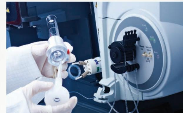
The user-friendly sample introduction system with push-fit connections ensures rapid assembly and disassembly for cleaning and maintenance. Alternative sample introduction components can be added to increase the speed of analysis or for the analysis of special sample types.
